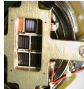
FLAPS qualification model: left showing close up of 5 detectors, right showing entire assembly
